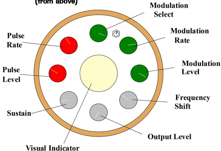
The effect the modulation signal has on the sound is increased by clockwise rotation of the *Modulation Level* control.
