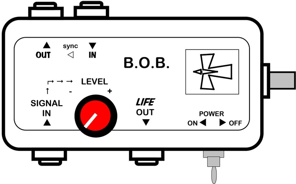
*BOB* is the **Break Out Box** used to interface *LIFE* to some aspects of the outside world. *BOB* also houses a *Power* switch to turn *LIFE* on and off without the need to remove the connector from the base of *LIFE*.
